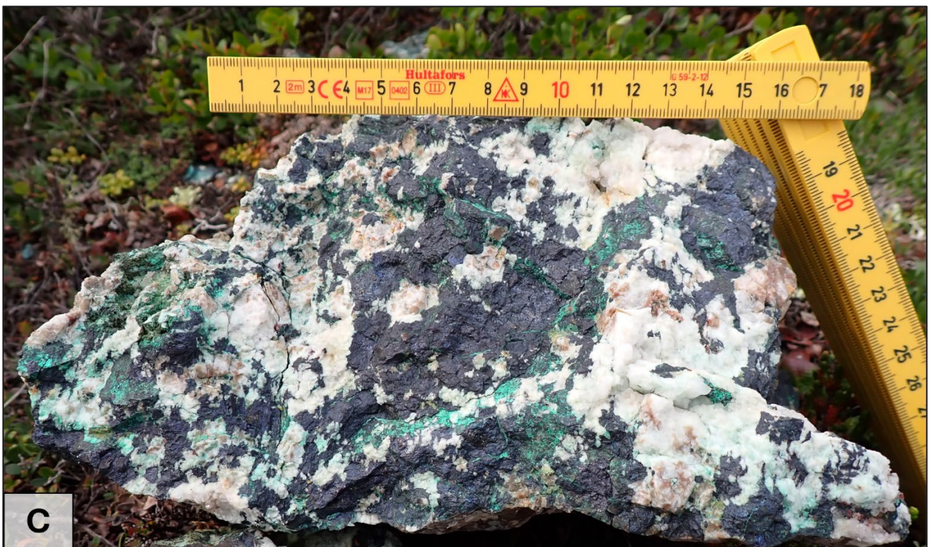
Figure 10 - Examples of the varying mineralisation styles at the Rae Cu-Ag-Au Project. A) chalcocite-chrysocolla-malachite-cuprite-native copper mineralisation within a vesicular basalt at the Kilauea Target. B) Chalcocite replaced bedding planes of a sandstone at the HALO Target. C) Coarse grained chalcocite within a quartz-carbonate vein at the PAT Target with secondary malachite-chrysocolla.
