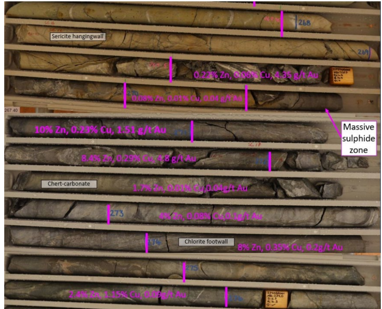
Leonora VMS discovery hole IP22DD001. Marked massive sulphide interval between 270.3m-276.0m graded 5.3% Zn, 40 g/t Ag, 1.0 g/t Au, 0.3% Cu and 0.3% Pb see ASX:KIN release 'High-Grade VMS Mineralisation Discovered at Cardinia East' 8 January 2024 for details.
