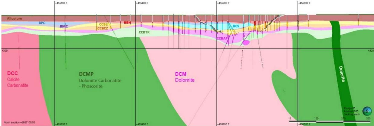
**Figure 4: North section 6807105mE lithological and mineralogical domains at Mt Weld**
