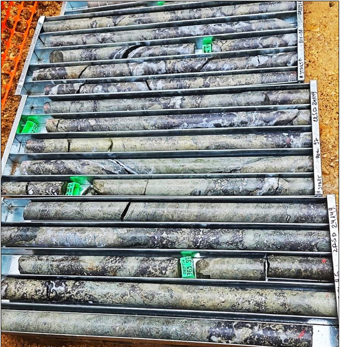
Figure 7. Core box photos from ZRSD24149 showing extensive sulphide mineralisation, including massive chalcopyrite within magnetite skarn
