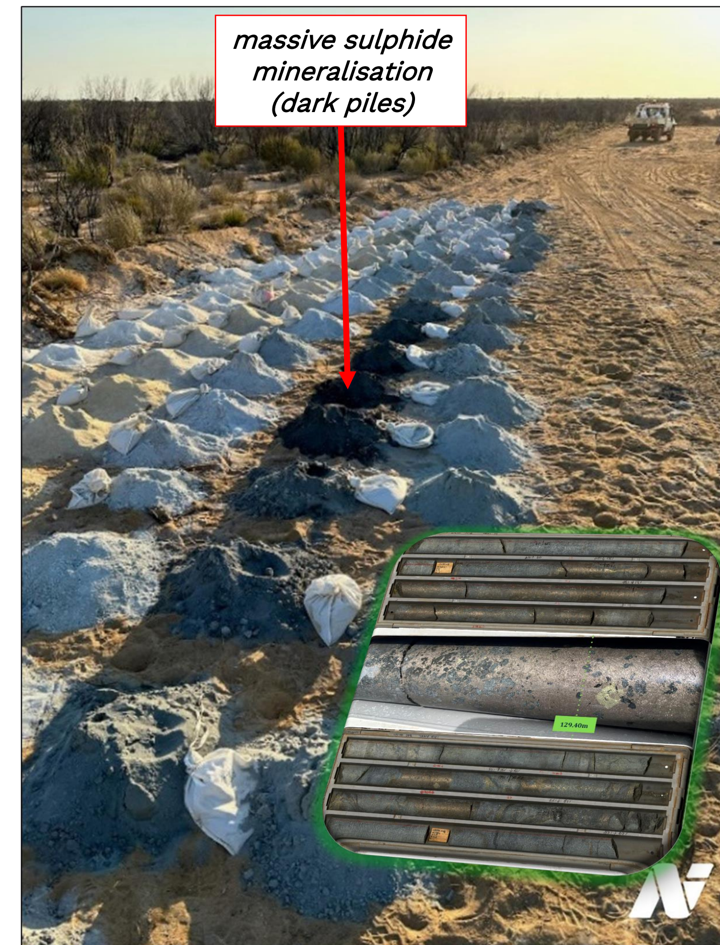
Masson Prospect discovery drill hole NRRC0100 showing Massive and disseminated sulphide mineralisation (5m @ 0.73% Ni, 0.53% Cu, 0.06% Co and 0.55 g/t 2PGE from 102m). Inset of follow up diamond core (massive sulphides)
