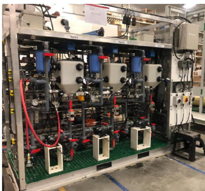
Figure 3: Pilot Scale Lithium Carbonate and Wash Equipment
