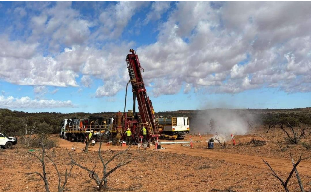
Figure 1: Photo of the Topdrill RC rig drilling at the Stinger niobium target.
