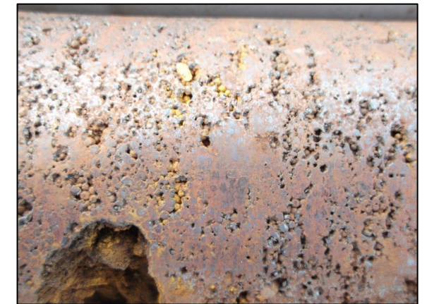
Cemented pisolitic detrital (PZ) comprising fine hematitic pisoliths with a cemented matrix of goethite and hematite
