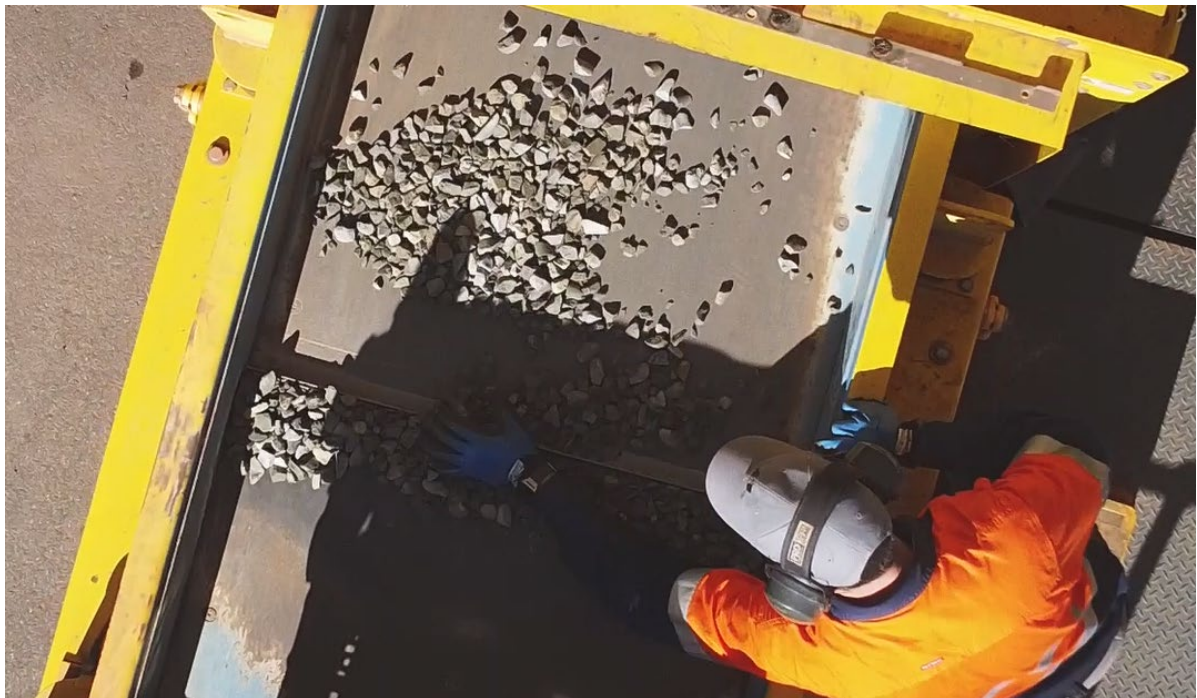
Figure 1: Storm copper mineralisation being processed by a full scale Steinert ore-sorter in Perth, Australia.
