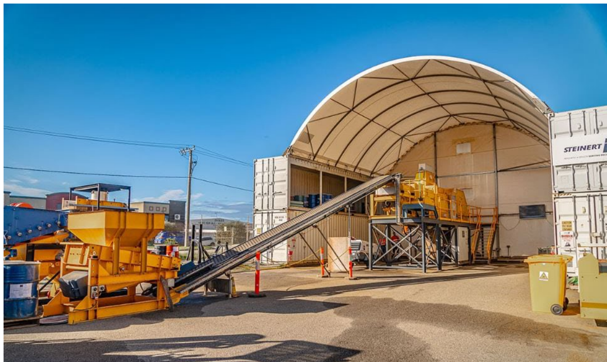
Figure 12: Photo of a Steinert KSS KLI XT ore sorter and feed bin. Source – Steinert.
