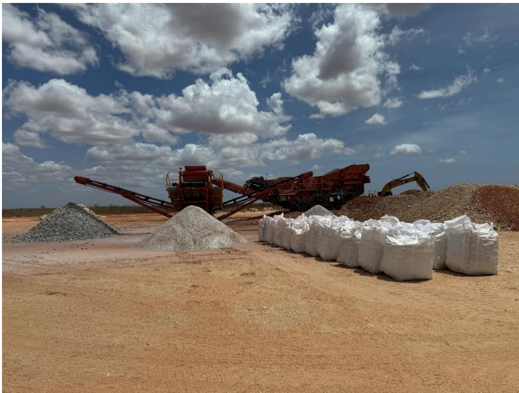
Figure 4: Crushed, screened, and bagged raw quartz samples prepared for further HPQ testwork.
