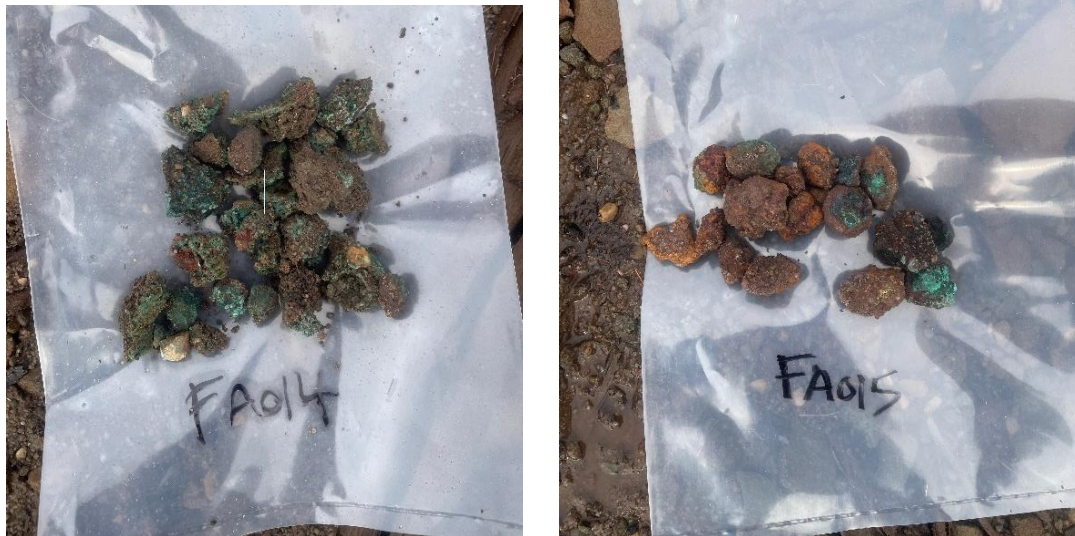
Figure 2. Photos of rock chip samples from Tantramar. Assay results in Appendix 1. Left: Sample FA014 = malachite/chalcocite bearing gossans collected from supergene zone Assay result = 30% Cu, 53 g/t Ag. Right: Sample FA015 = similar lithology/mineralogy to FA014. Assay = 38.4% Cu, 151 g/t Ag
