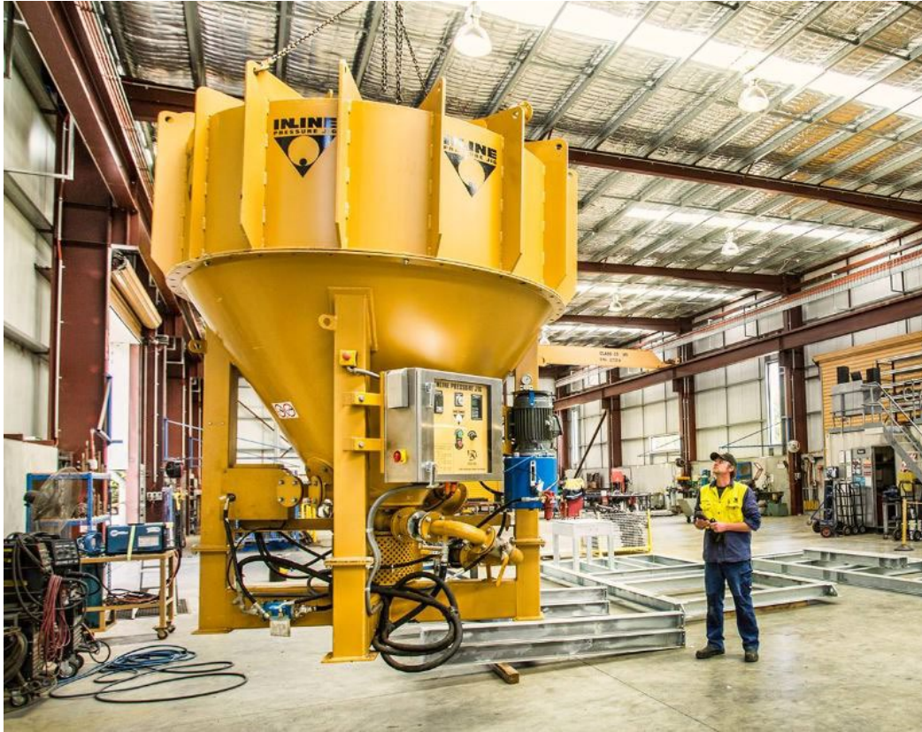
Figure 13: Photo of a Gekko Inline Pressure Jig (IPJ). Source – Gekko.
