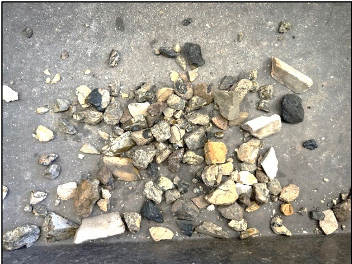
Figure 4: Photo of a high-density cut using XRT ore sorting of -26.5/+11.2mm low-grade composite material. This sample returned a grade of 15.2% Cu from a feed head grade of 0.78% Cu. Note the dark grey/black particles which are chalcocite (copper sulphide), veinlets of chalcocite within most of light grey host rocks (dolomite).
