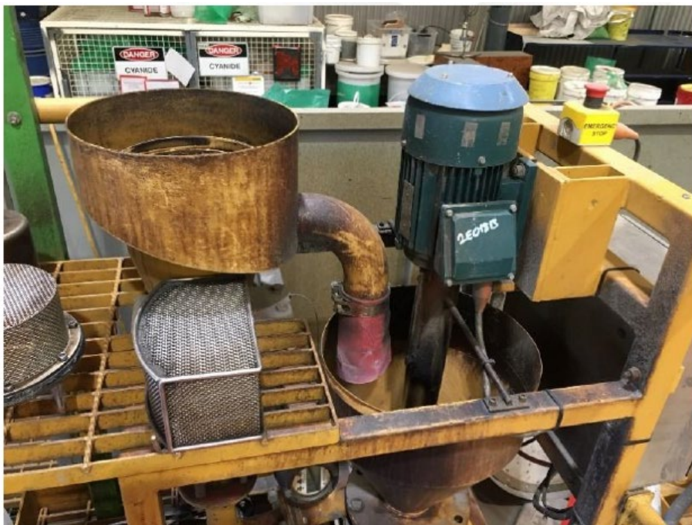
Figure 6: Dense Media Separation (DMS) Viking Cone at the Gekko laboratory.
