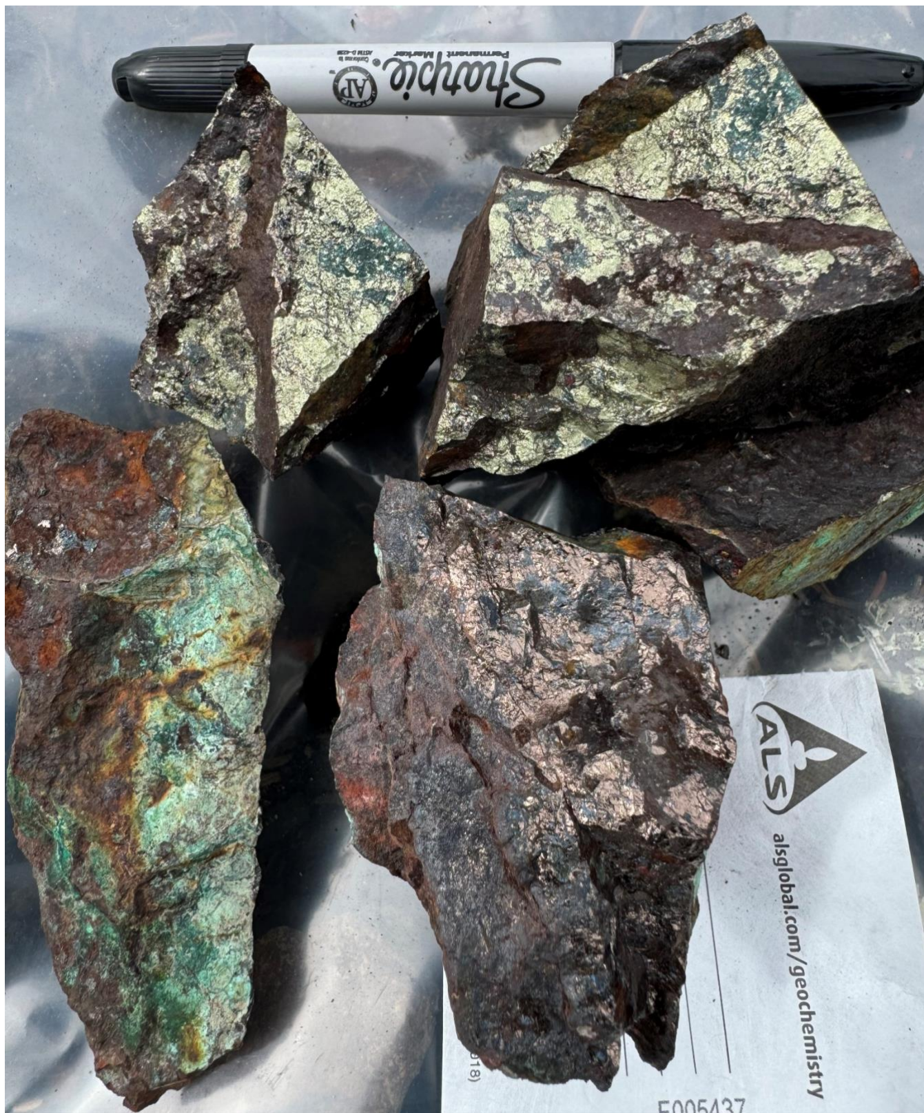
Figure 2 – Photograph of sample F005437 with massive bornite-chalcopryite which returned 42.60% Cu, 2.28g/t Au, 159g/t Ag, 0.364% Co from the Glacier IOCG trend.
