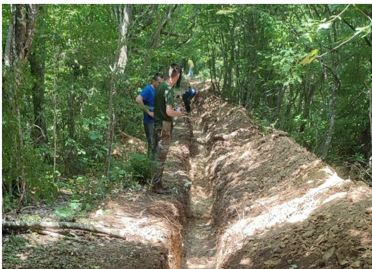
Figure: Trenching and channel sampling along old forest tracks (note the shallow trench depth due to thin soil cover)
