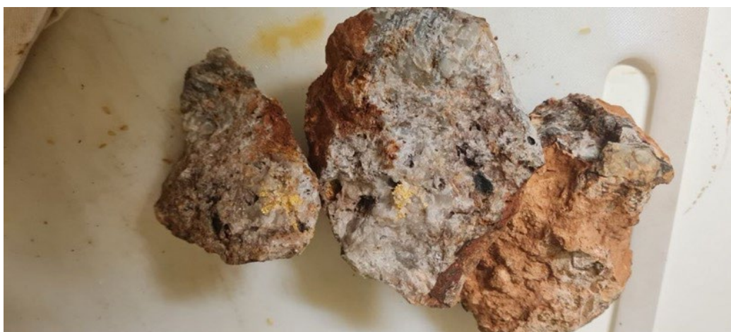
Figure 21 Abundant coarse gold observed in surface quartz veining chip samples (24AR11-013) collected from Titan Prospect
