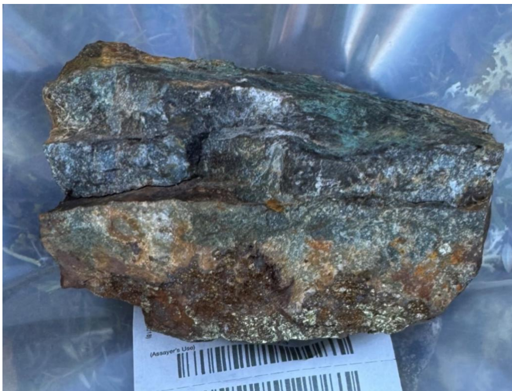
Figure 3 - Photograph of sample F005669, quartz-sulphide veining from Coyote which returned 16.95g/t Au, 45.3g/t Ag and 10.55% Cu .
