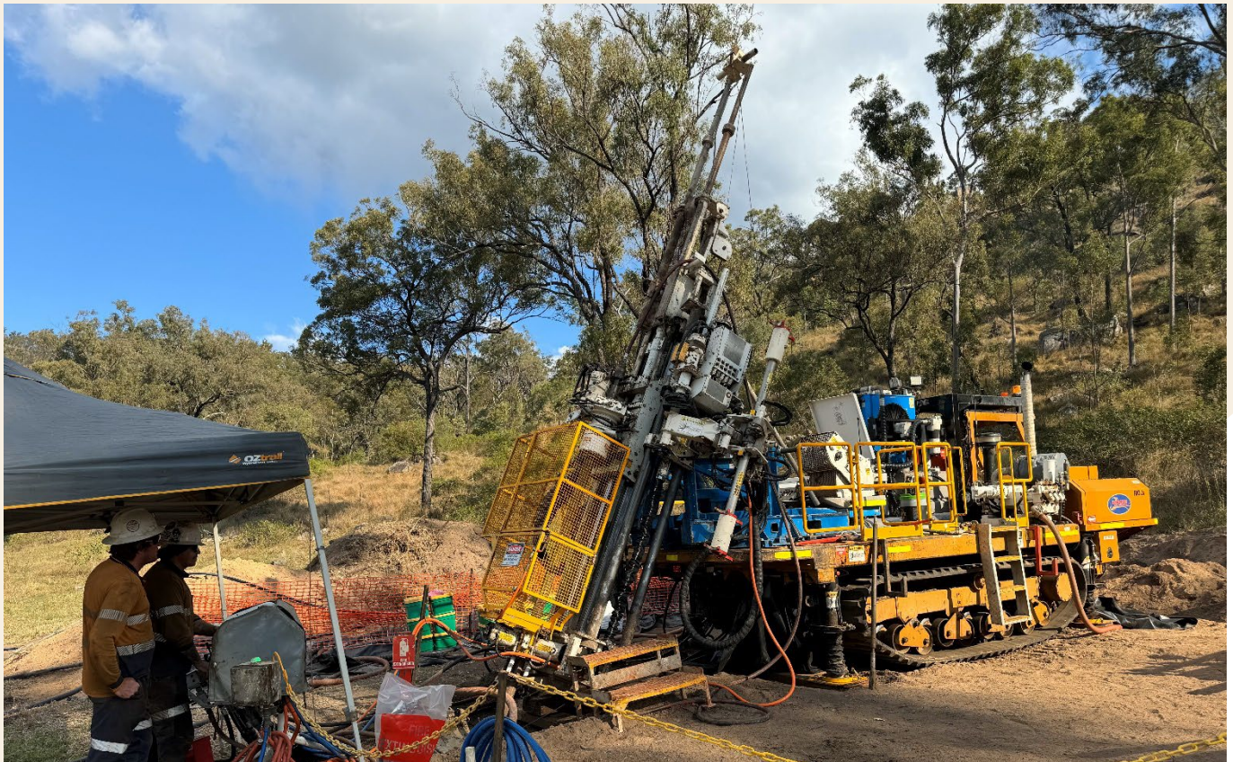
Figure 1. Diamond drill rig at the Kaa target, on planned hole PDH001, with Deepcore Drilling.
