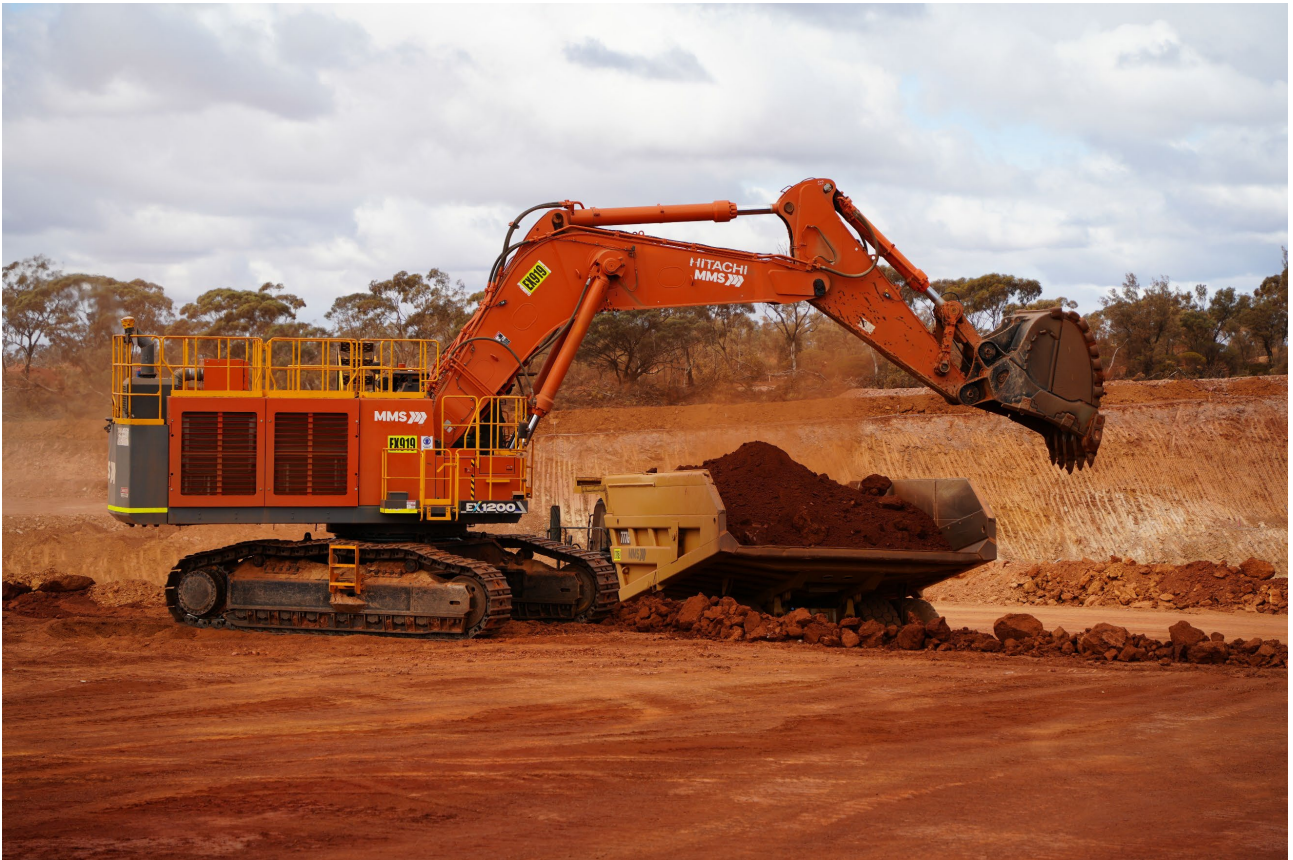
Figure 2: New 100t excavator conducting low cost, free-dig operations in the Myhree open pit
