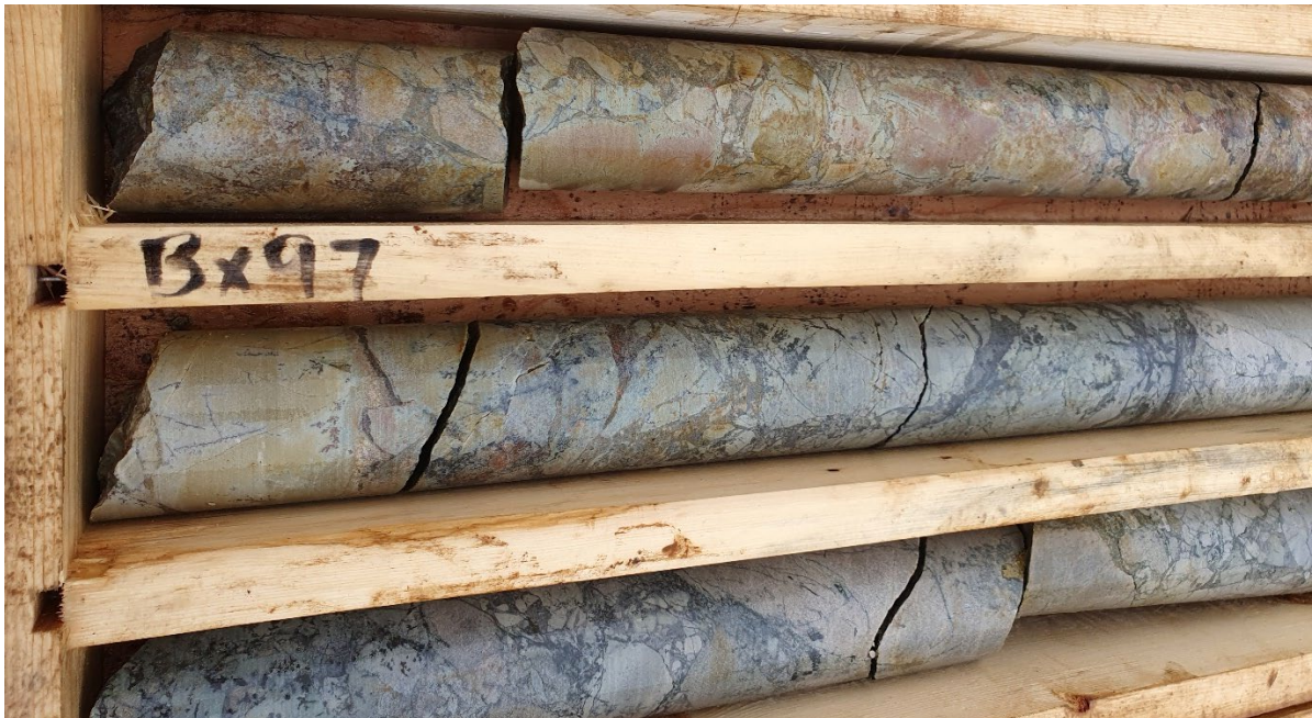
Figure 1: Drill core from ST24-01 from approximately 315.4 – 318m downhole. Dense veins and breccia of visible chalcocite (copper sulphide) can be seen as dark sooty grey, within light grey/mustard dolomite host rocks. This interval also contains blebs of native copper (brassy gold).
