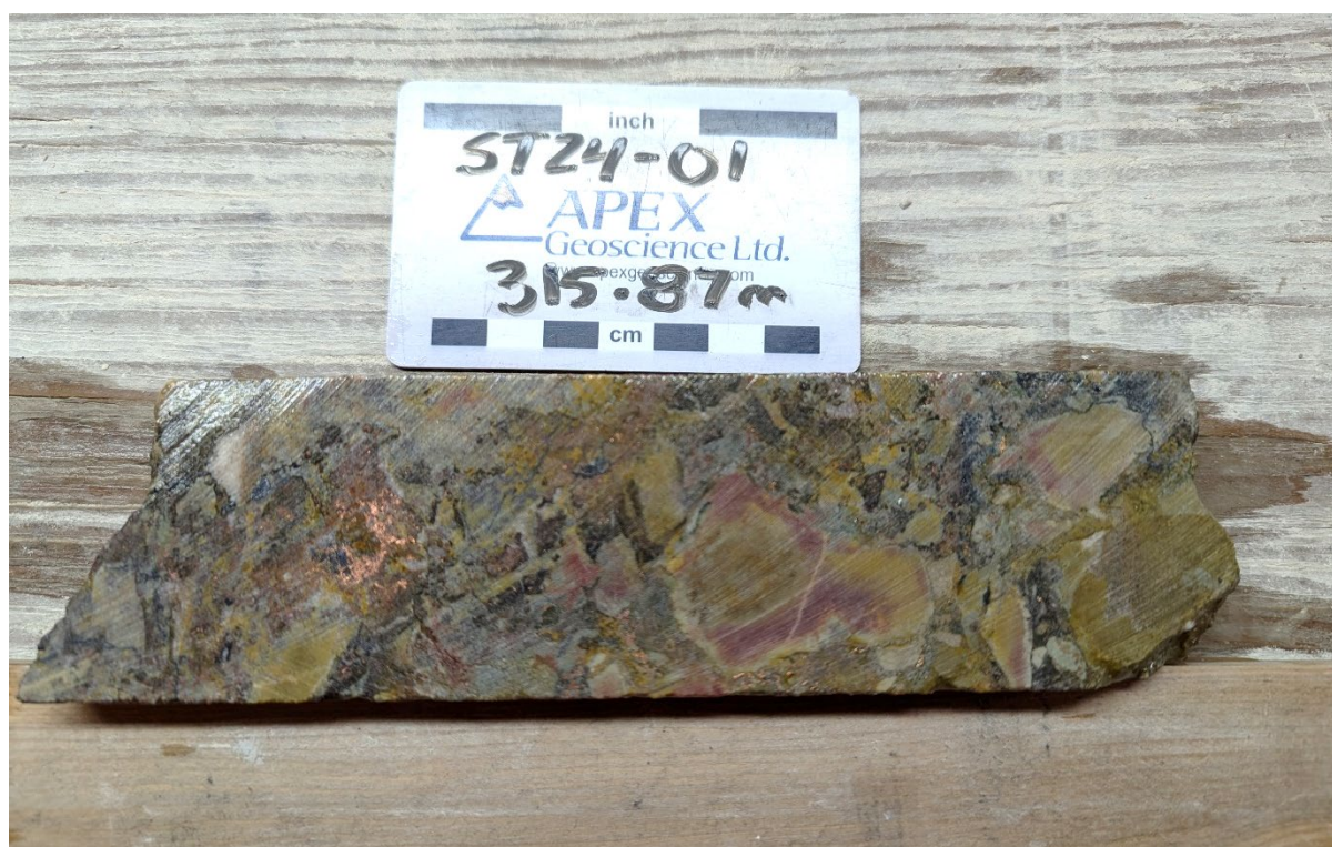
Figure 3: Chalcocite (dark grey) breccia and native copper (brassy) blebs within fractured dolomite in drill hole ST24-01 from approximately 315.87m downhole.
