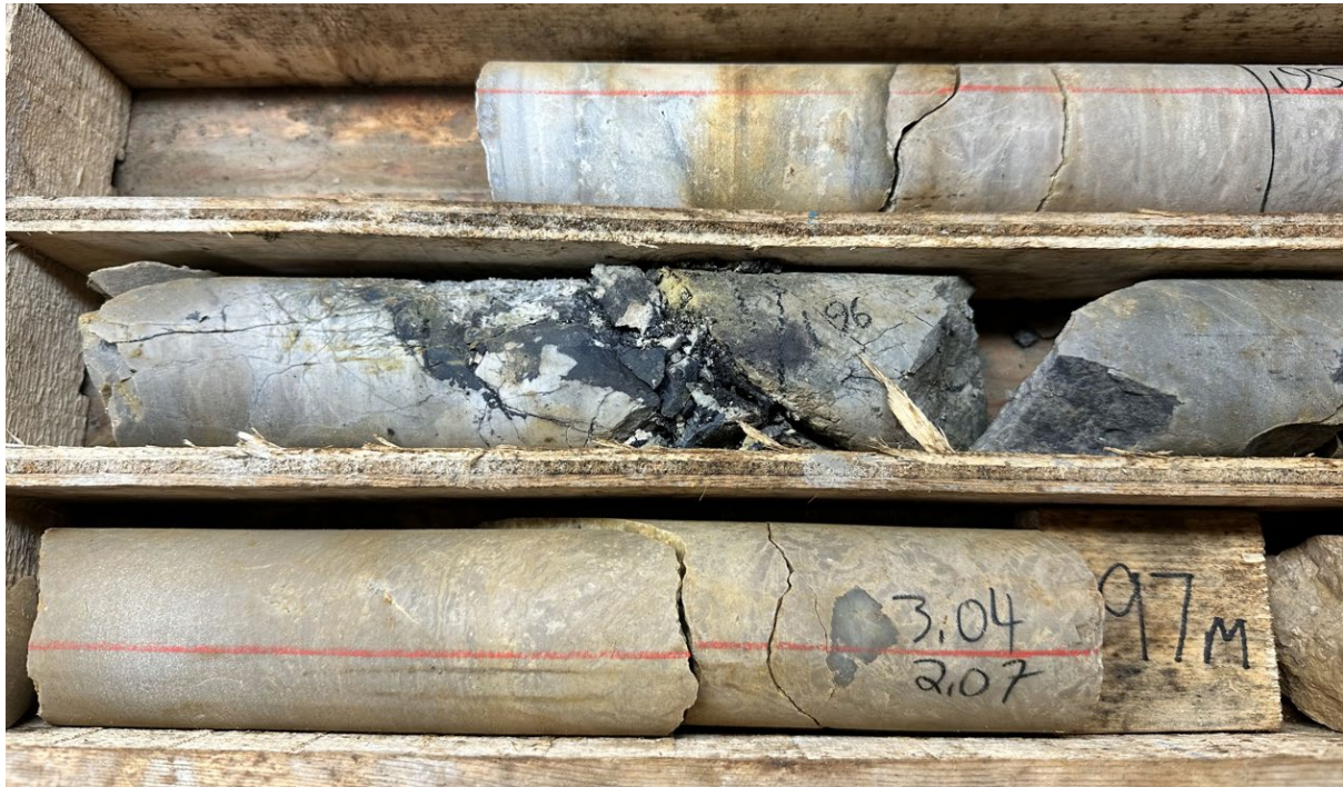
Figure 5: Chalcocite (dark grey) fracture fill in drill hole ST24-02 from approximately 196m downhole.
