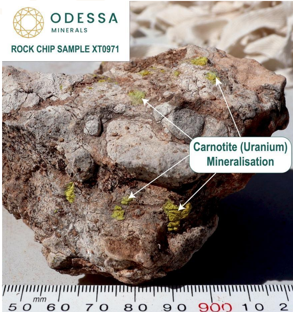
Figure 5: Uranium-bearing carnotite mineralisation in rock chip sample XT0971 at the Baltic Bore prospect.
