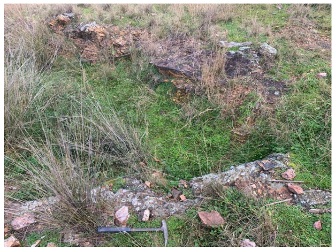
Unnamed old workings near sample location GRR255 and site of drill hole JUN016. The lode dipped west and has a strike of 15°-195° enabling an optimal azimuth to be determined for hole JUN016.
