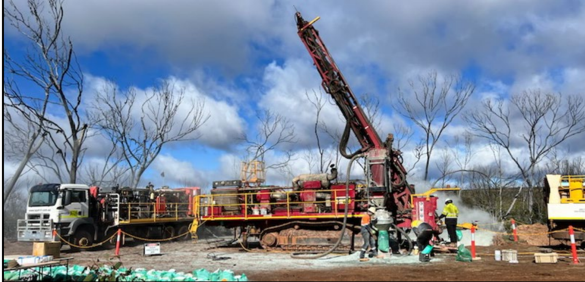
Fig 1: RC drill rig on site at the Norseman Project
