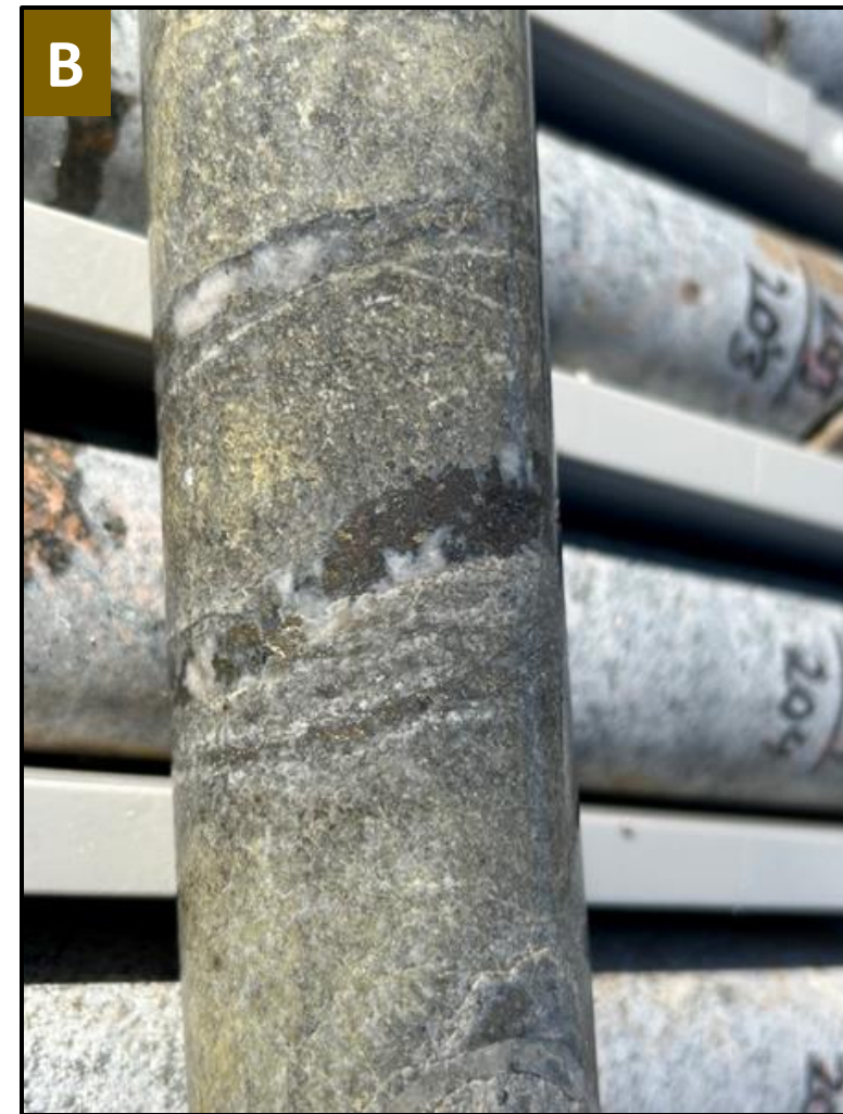
ZMRDD052 -213m, brown (Fe-rich) sphalerite in an extension vein, surrounded by disseminated pyrite (1m @ 1.1 g/t Au, 29.9 g/t Ag)
