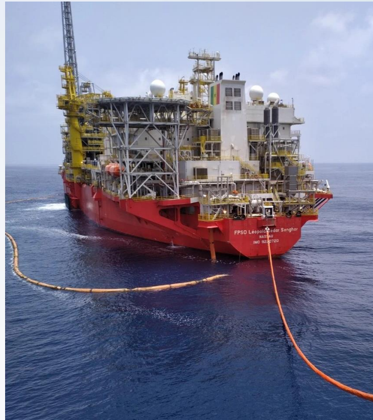
Tanker offload in progress
