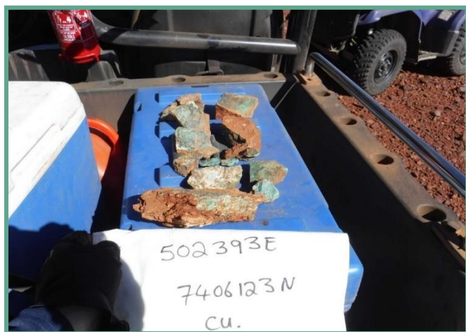
Photo 1 & 2: Photo 1, Rock chip sample SCR9 with 1% Sb, 30.2% Cu and 151g/t Ag from Station Creek Project (Photo 2.).
