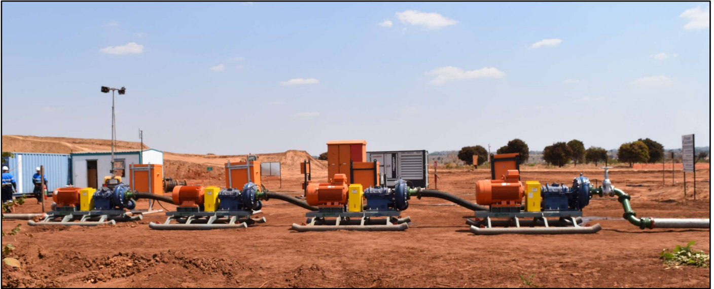
Figure 4: The train of high-pressure pumps used to drive the water monitor are skid-mounted.
