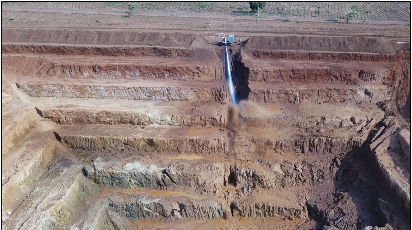
Figure 1: Hydraulic mined material (slurry) flows freely to the collection point in the bottom of the sump.
