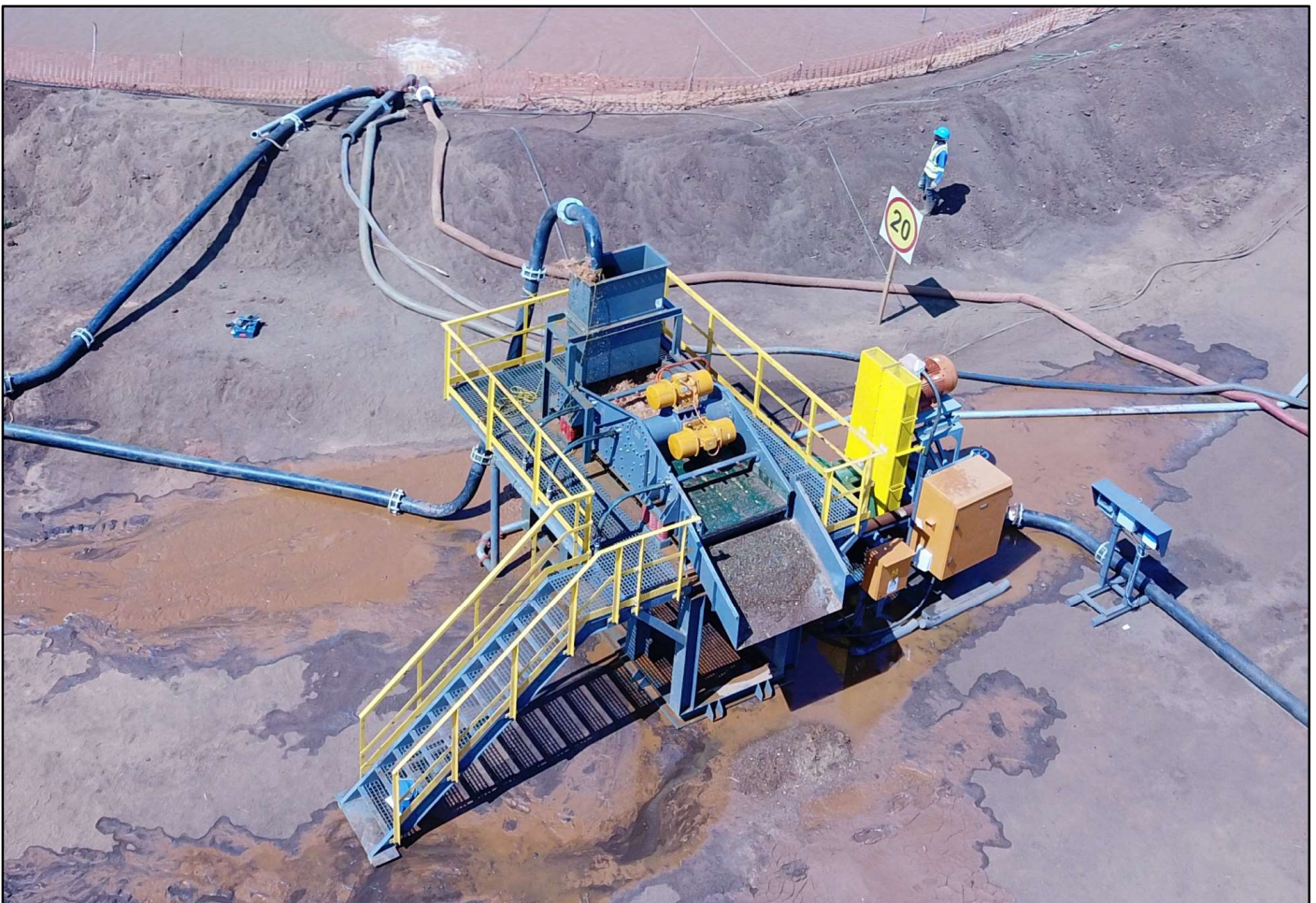
Figure 5: +2mm oversize is screened out using a vibrating screen.
