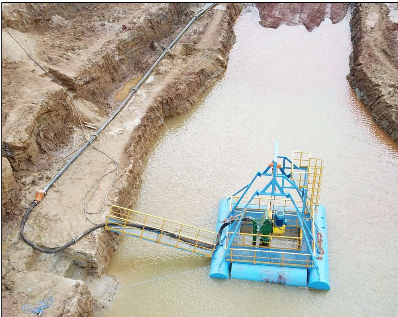
Figure 3: A pump, mounted to a barge, pumps the slurry to a vibrating screen.
