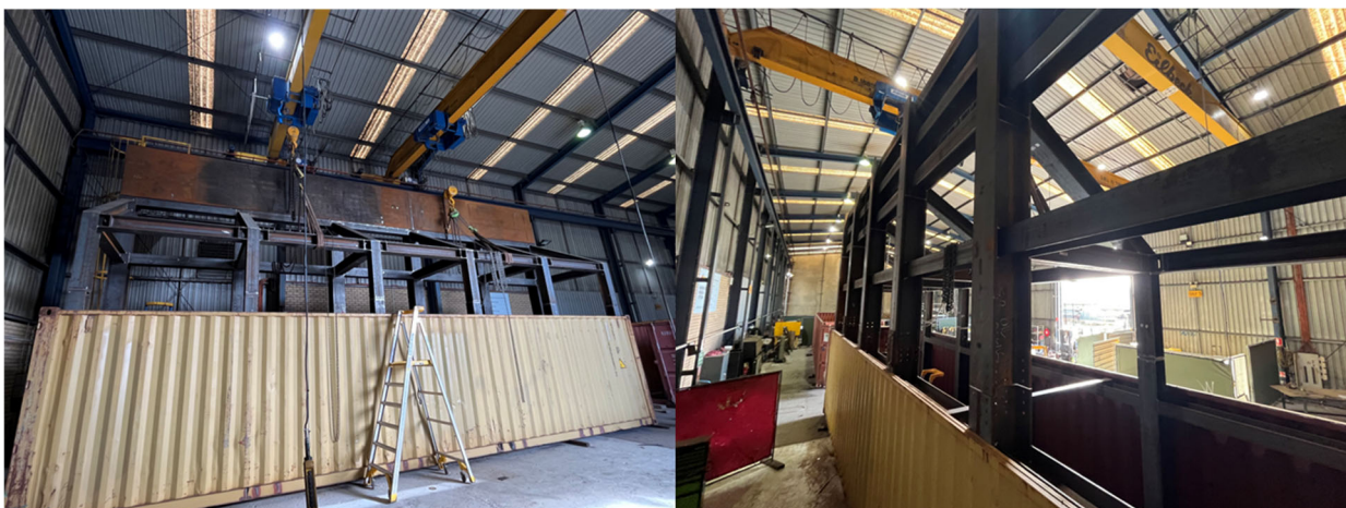
Figure 2: ROM wall fabrication, now complete and ready for installation.
