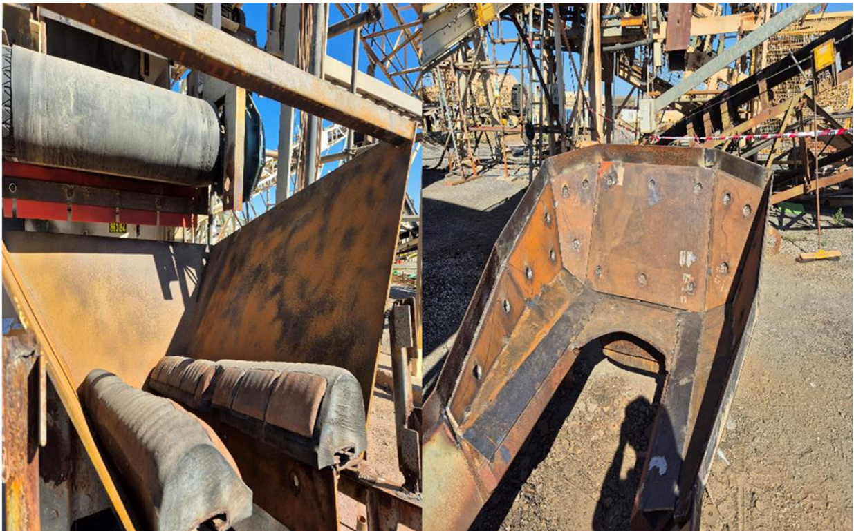
Figure 4: Chute repairs in the crushing circuit.
