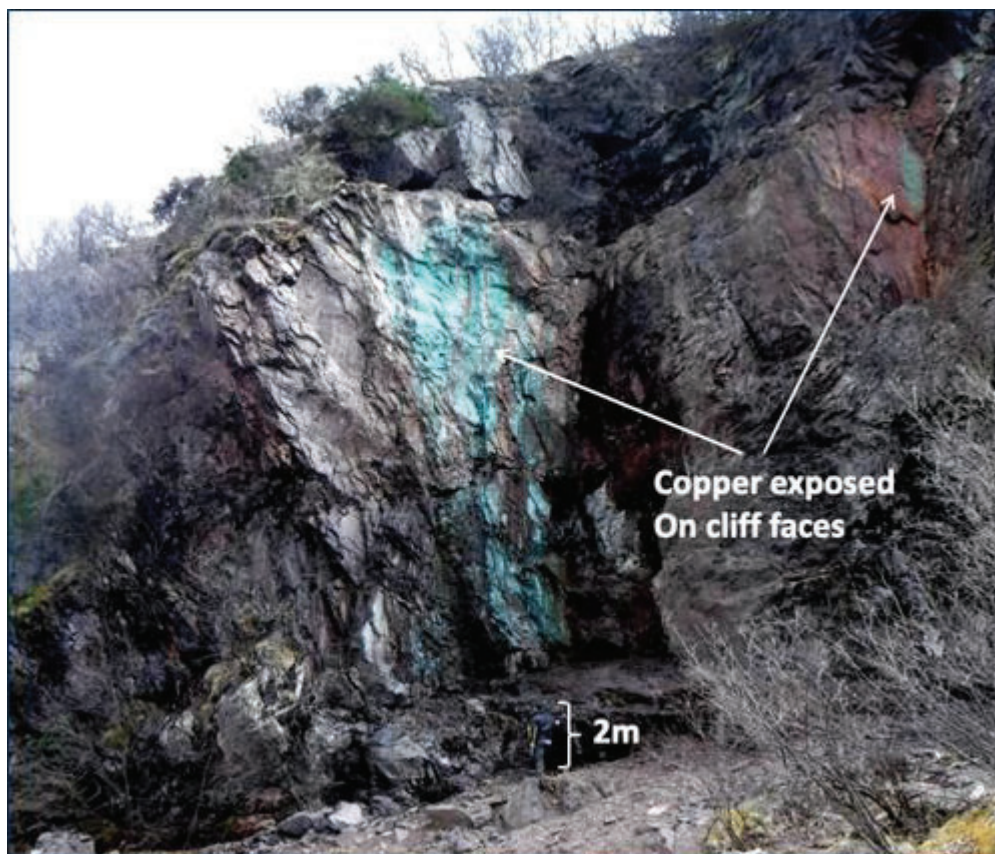
FIGURE 5: HISTORICAL SAMPLING RETURNED 2.15% Cu, 1.5% Cu, 0.9% Cu AND 0.7% Cu IN CHALCOPYRITE, CHALCOCITE, BORNITE, MALACHITE AND AZURITE 8
