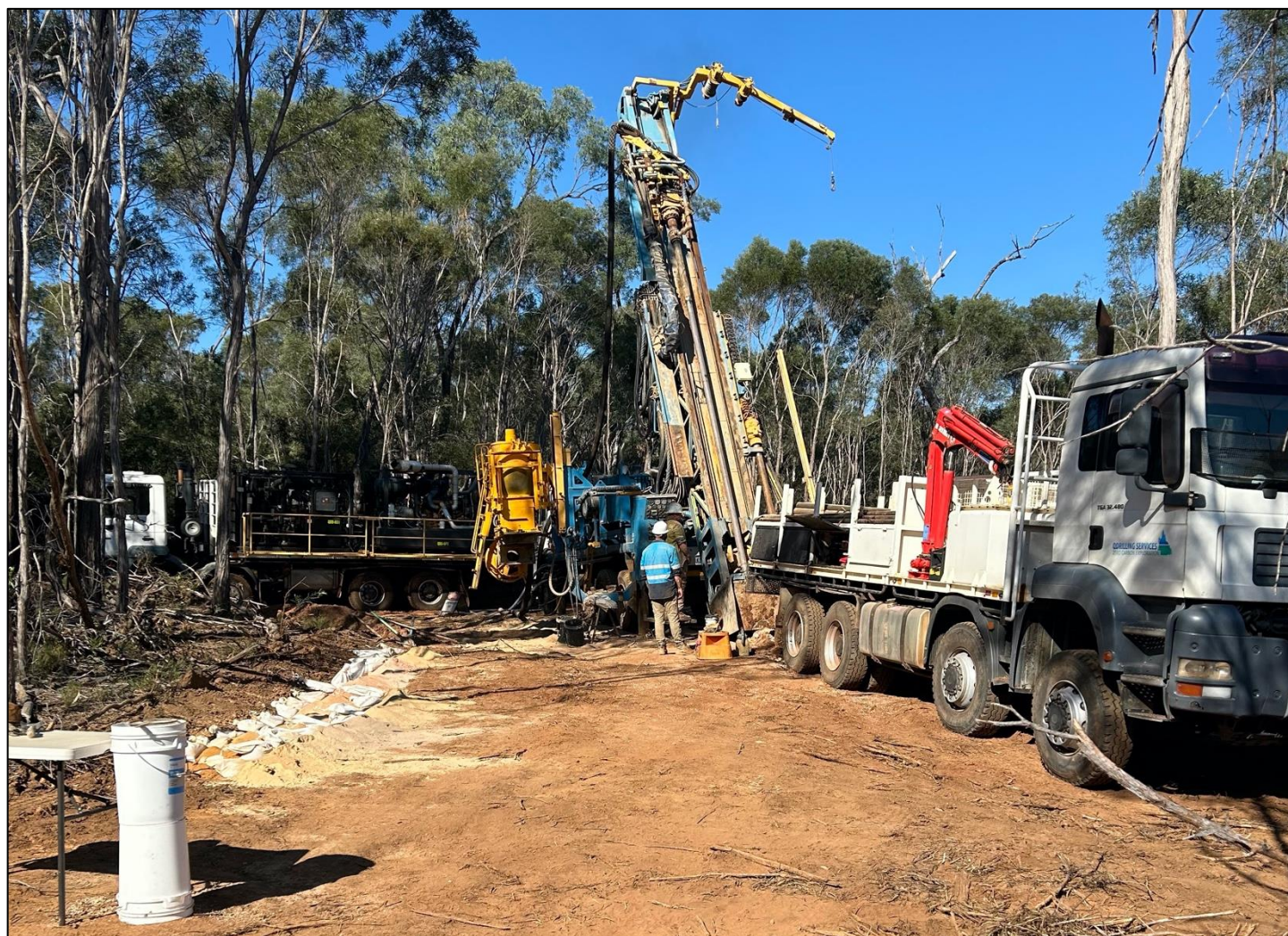
Figure 2: QMines RC rig operating at the Develin Creek copper project.
