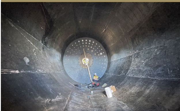
Laverton mill re-start - Ball mill relining
