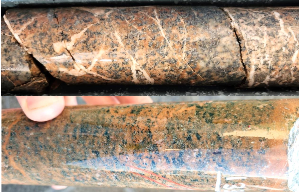
Figure 4: Examples of hematite dusting of feldspars: with carbonate veining at 873m (top) and with pervasive hydrothermal pyrite at 1,333m downhole.
