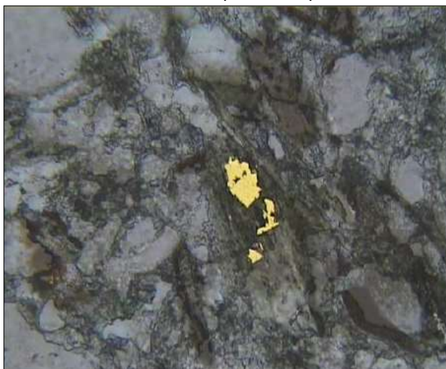
Photo 1: Thin section from 24ATAC023 (135-136m), showing fine-grained chalcopyrite intergrown with hydrothermal biotite, alkali feldspar and sericite. The photo is 0.6mm wide, under plane polarised light.
