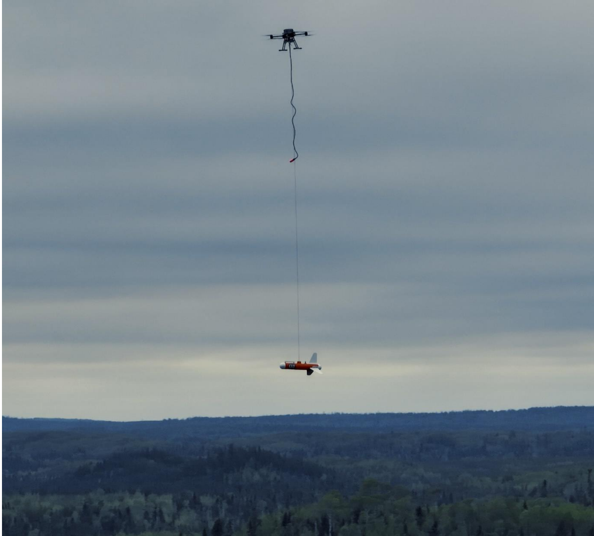
Figure 1. Photograph of drone VLF-EM and magnetics survey in progress. Note: Image is not from FMR's project. (Source: Pioneer Exploration)
