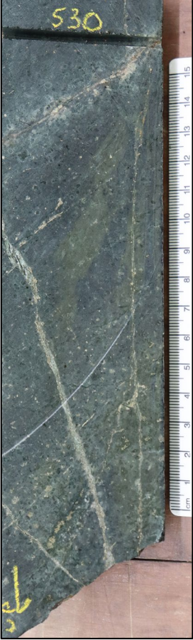
NCG004 529.9m chl- altered pyroxene porphyry with pyrite+chalco+qtz veinlets
