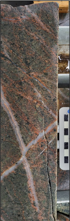
SD003 82.5m hornblende-K-feldspar- plag monzodiorite porphyry
