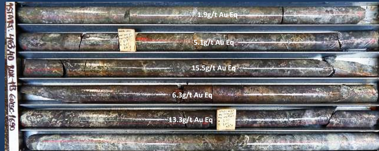
High-grade Copper-Gold mineralisation in EOKSC1690 –Shanac deposit
