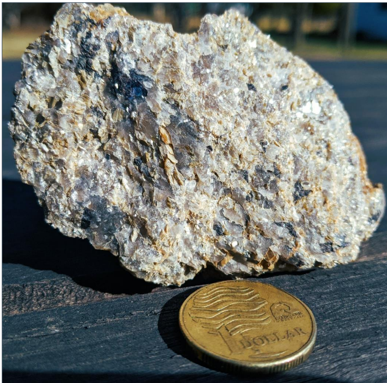
Figure 3. Numerous dark cassiterite grains in quartz vein from McLurg's historical tin mine
