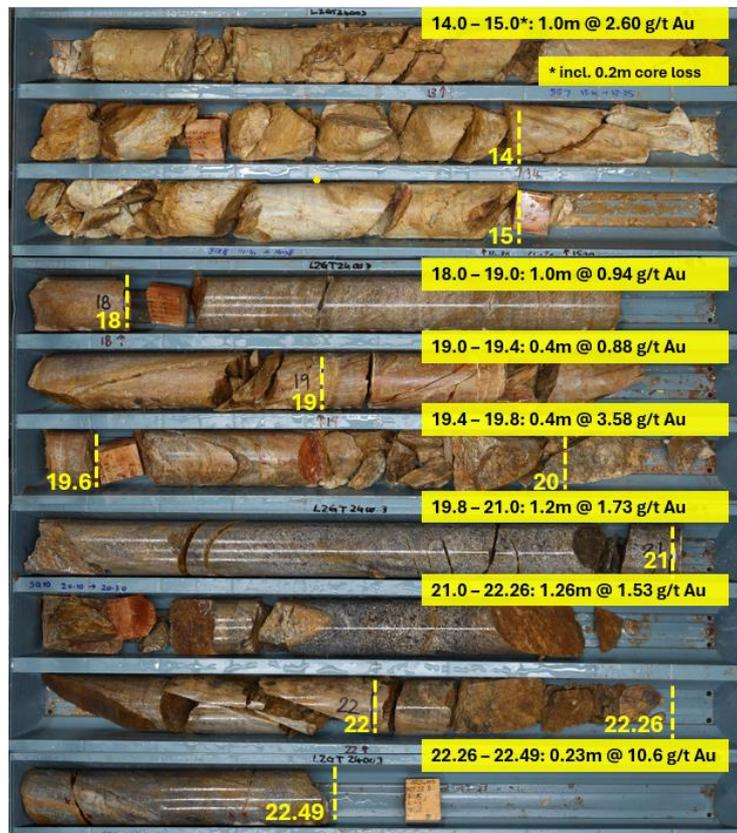
Figure 4 - LZGT24003 Tray 6 (upper 3 rows) and Trays 8-10 (lower 7 rows) displaying typical Link Zone oxide/transitional mineralised zones within broader 8.49m @ 1.56g/t (from 14m) intercept at Merriyulah
