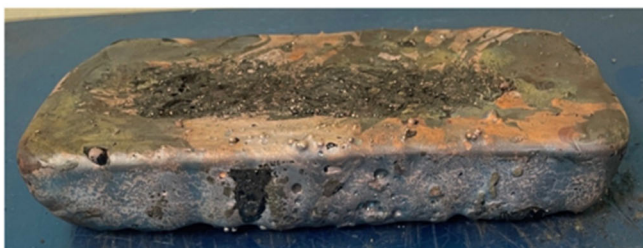
Figure 11: Doré bars produced from carbon stripping.
