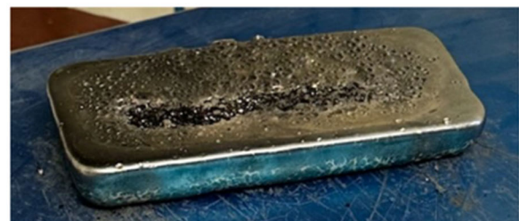
Figure 11: Doré bars produced from carbon stripping.
