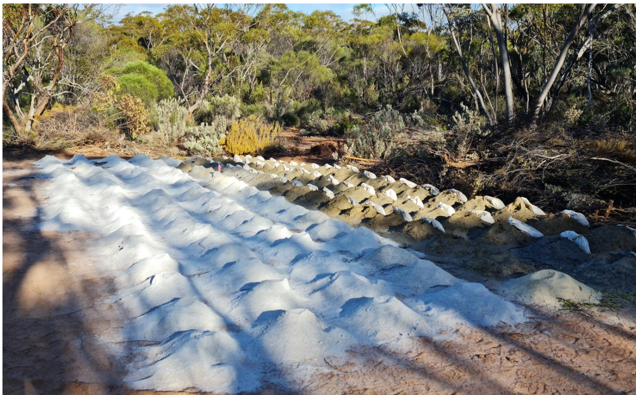
Figure 2 – Pegmatite intercept in NDRC04 from 67m to 152m (85m) down hole.
