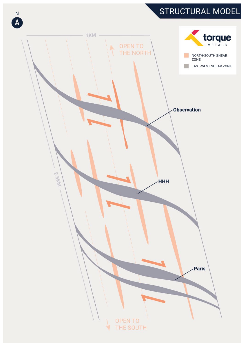
Figure 7 Schematic representation of the geological structures governing Paris, HHH and Observation deposits.
