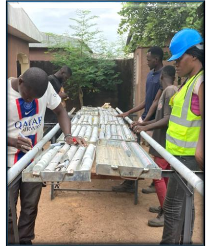
Figure 5 | Odienné Project diamond core processing – oriented core
