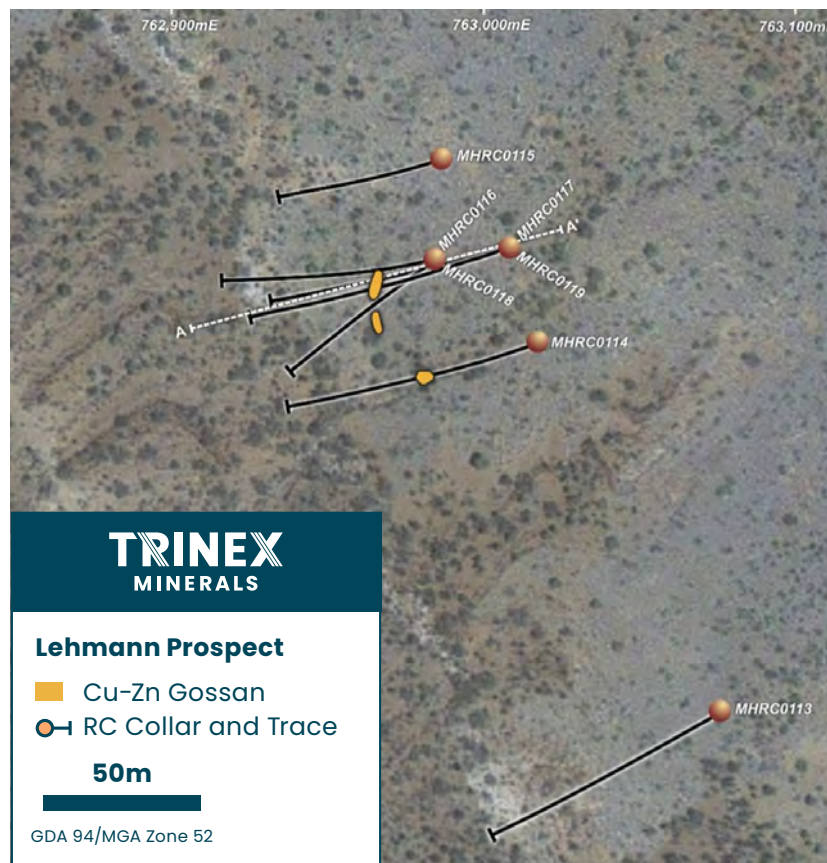
FIGURE 12: Collar plan for September 2023 RC drilling at Lehmann Prospect
