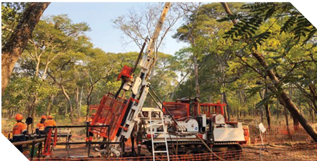
**Figure 5. Phase 1 Diamond drilling rig on site at the Mumbeshi Copper Project**
