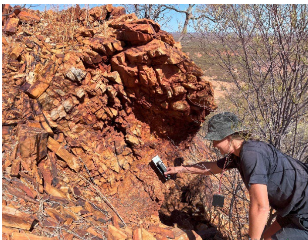
Photos 1-2: Field photos showing senior geologist Alex Forster (left) using a scintillometer to vector toward units of interest for sampling.
