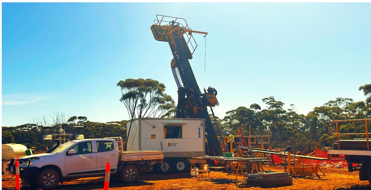
Image 2 – Diamond drill rig at Kamperman (November 2023).
