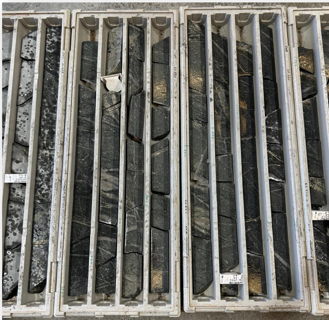
Figure 9: Photograph of core from BHRC030, 123m showing quartz-pyrite veins \pm chalcopyrite-molybdenum
