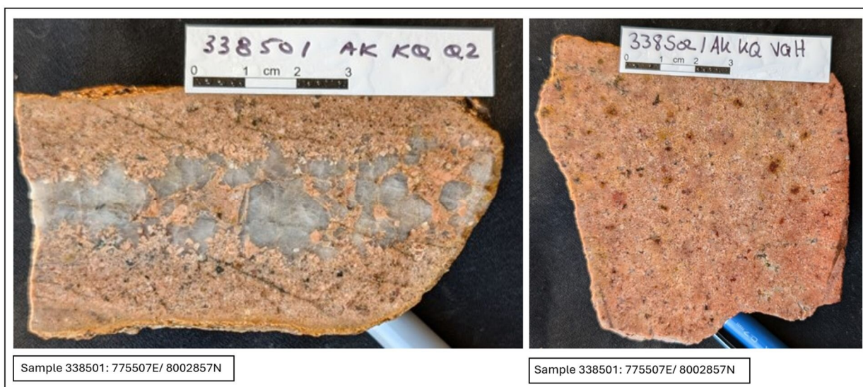
Plate 1: Sample 338501: Intrusive stock immediately to the south of the Fiery Creek Copper Prospect showing miarolitic cavities with goethite (dark orange, brown) after sulphides and a feldspar + quartz vein which equates to “brain rock” developed in the cupola of porphyry type systems such as Kidston.
