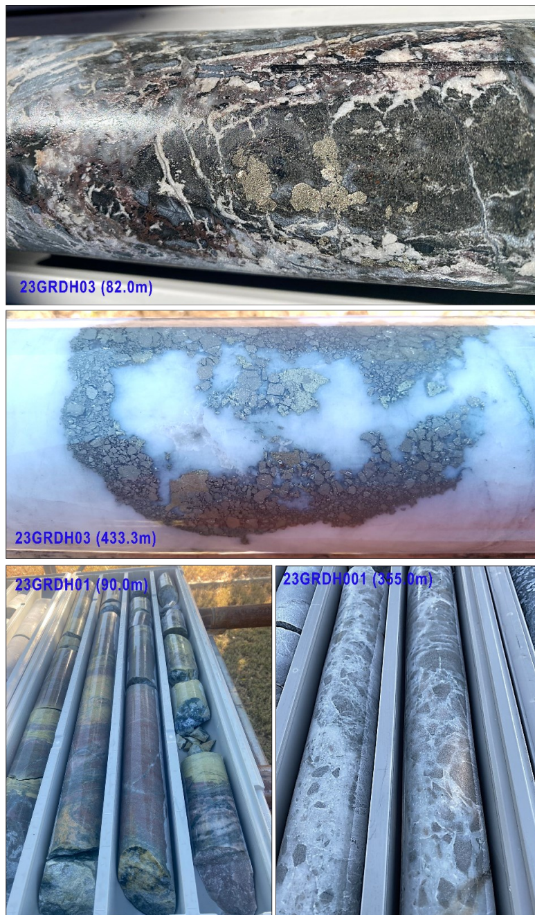
Figure 9: 23GRDH03 (82m): brecciation and sulphide infill of basalt; 23GRDH03 (433.3m): 400mm quartz-carbonate vein with early pyrite with later chalcopryite; 23GRDH01 (90.0m): Strong epidote-silica-hematite alteration; 23GRDH001 (355.0m): large zones of brecciated quartz-dolomite veins with trace sulphide (pyrite).
