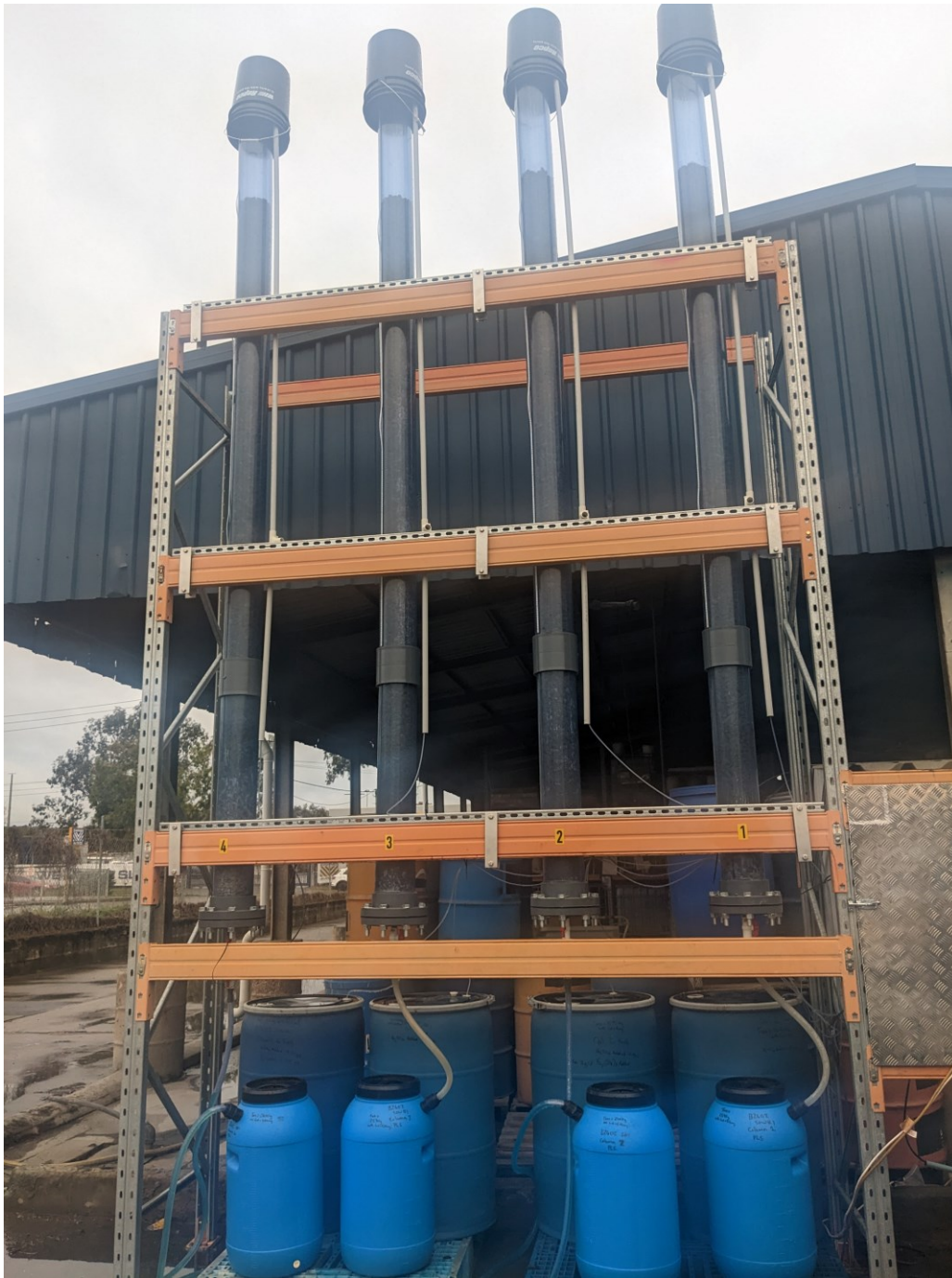
Figure 4: Column leach test work on the Dianne Copper Deposit material in progress
