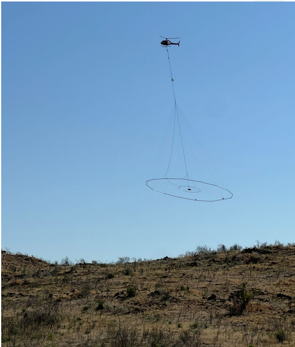
Figure 2. Helicopter VTEM survey in action at Mohawk.
