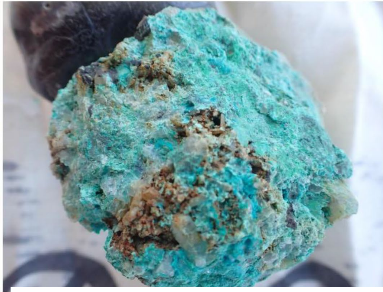
Sample ESS02045 - A white, frosty to glassy quartz vein hosting abundant drusy cavities lined with euhedral prismatic quartz crystals encrusted with supergene malachite and chrysocolla developed over sooty tenorite (Coordinates Location 774873E 8007987N)
