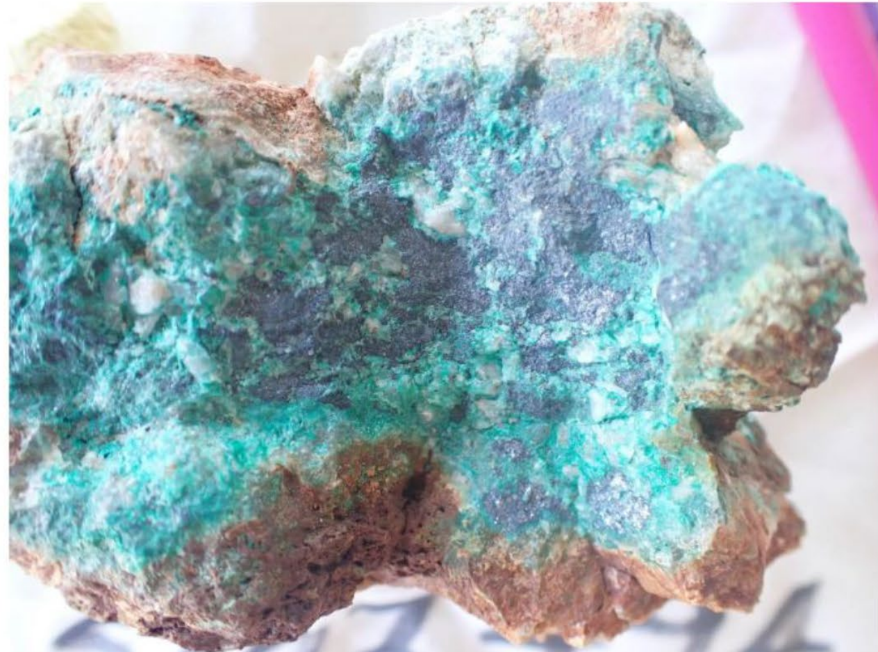
Sample ESS02494 – (460ppm Ag, 1.25% Ba, 23.51% Cu, 14ppm In). White frosty quartz vein invaded by a later massive sulphide event as a mix of black tenorite ( CuO ) and sooty to dark grey chalcocite ( \text{Cu}_2\text{S} ) replaced at its margins by crystalline fibrous malachite and minor chrysocolla (Coordinates Location 773511E 8007365N).
